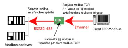
• Or a fixed address configured in the gateway (see below); in this case, only one slave can be addressed on the serial link.
