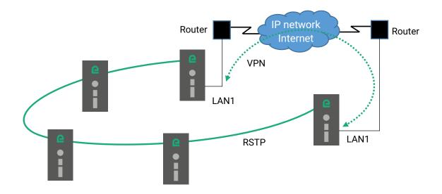
The 2 XS switches at the end of the network establish a VPN over the WAN. The VPN provides connectivity at the Ethernet level. Thus by activating the RSTP protocol redundancy may be provided thanks to that VPN.
