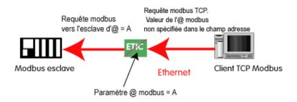
**Warning :** Several TCP Modbus client can send requests to the slaves on the serial link. Nevertheless, care must be taken not to saturate the serial link since its flow rate is much lower than the Ethernet one.
